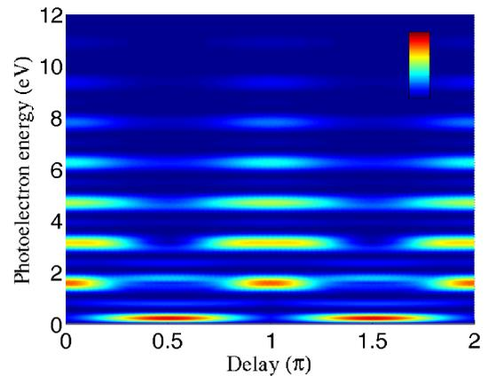
**Fig. 1.** Photoelectron energy spectrum for  $I = 1.3 \times 10^{13}$  W/cm<sup>2</sup>, 6 IR cycles and 2 atto pulses per cycle [4].
