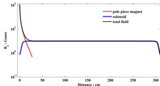
Fig. 1. Calculated magnetic field along z-axis ( $B_z$ ).
