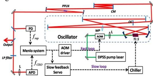
Fig. 1. Schematic of double feedback control for  $f_{CEO}$  locking.
