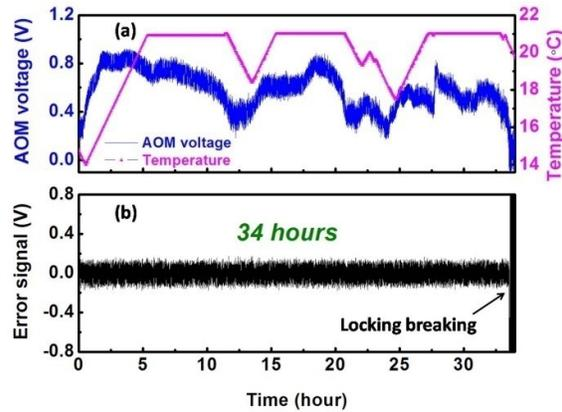
Fig. 2. (a) 34 hours CEP stabilization achieved by employing the double feedback loop; the blue curve shows the AOM driving voltage output; the pink curve shows the temperature of the crystal; (b) Error signal from locking electronics.
