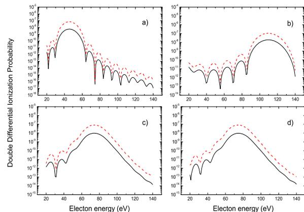
**Fig. 1.** Double differential ionization probability. Full lines: CVA. Dashed lines: SFA. a) Forward ionization with time delay. b) Backward ionization with time delay. c) Forward ionization without time delay. d) Backward ionization without time delay.
