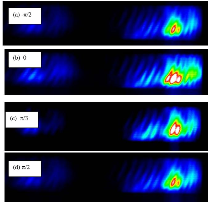
**Figure 1.** Measured XUV Spectrum from interaction of neon gas with CE-phase stabilized 5-fs laser pulse. (a)-(d) obtained for different CE-phase settings, by changing the insert of fused silica wedge
