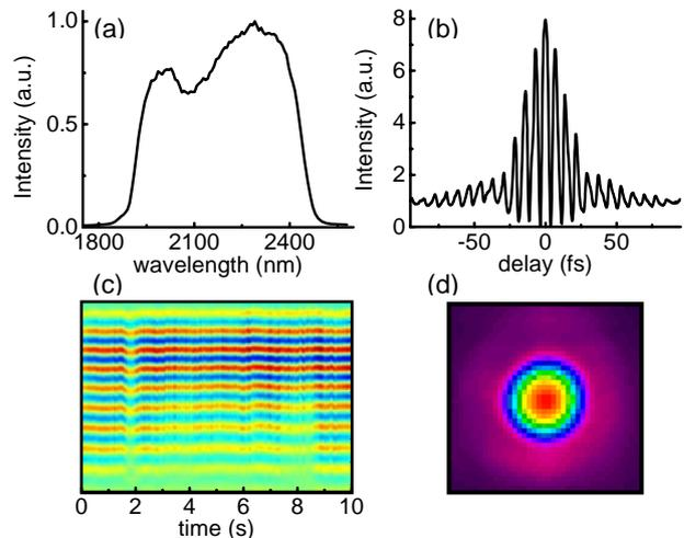
**Fig. 1.** (a) Amplified spectrum, measuring 500-nm FWHM in bandwidth. (b) IAC of the compressed pulse, measuring 23 fs (3 cycles). (c)  $f$ - $3f$  spectral interferogram, measuring 150 mrad rms in CEP fluctuation. (d) Pyroelectric CCD image of the output beam.
