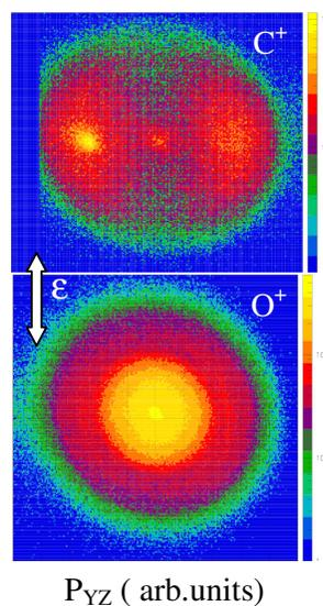
**Fig. 1.** Momentum image of the  $C^+$  (up) and  $O^+$  ions generated from the dissociation of CO by few-cycle EUV laser pulses. The polarization is vertical.
