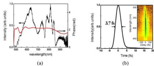
**Fig. 1.** (a) Spectral profile and phase of the laser output taken with 1.6-bar neon and positively chirped 33-fs laser pulse, and (b) temporal profile of the laser pulse measured using the SHG FROG method. The inset shows the FROG trace.
