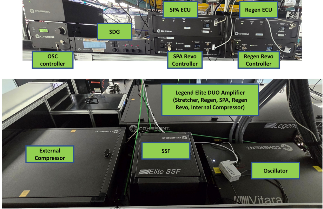
Figure 2.2: Physical layout and control hardware of the FLAME system. Major components include the Vitara oscillator with a CW pump laser (Verdi), the Legend Elite DUO amplifier, pump lasers (Revolution), enclosed Ti:sapphire regenerative (Regen) and single-pass amplifier (SPA) stages with environmental control units (ECU), internal and external grating compressors, beam-delivery optics, and synchronization and delay generator (SDG). See text for a brief description of each of these units. Controllers used for oscillator and pump-laser control are also shown.
