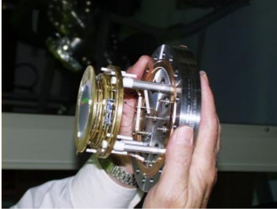
Figure 2. Recoil detector assembly showing the ground ring, grid, channel plate holder, the drift region and the position-sensitive backgammon board and holder.
